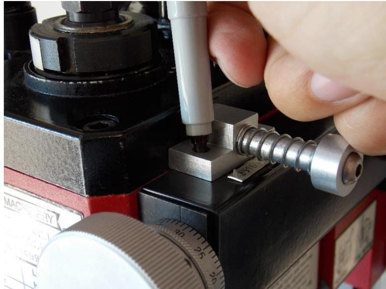
**3. Remove the fine feed cover by removing the two screws securing it to the head.**
